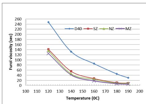
Fig. 5 Furol viscosity of WMAA
