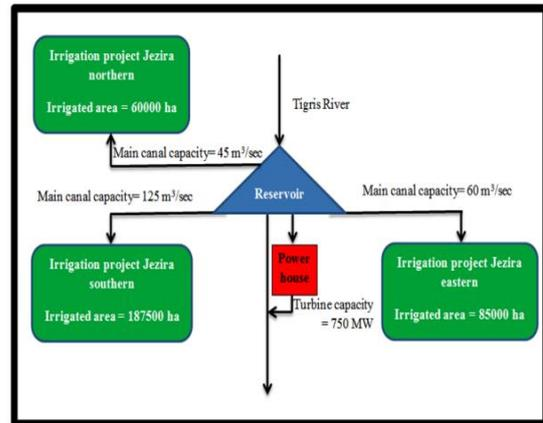
Fig.4 Schematic representation of multipurpose Mosul reservoir system
