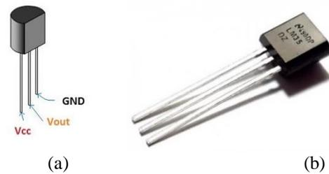
Figure 2: (a) Lm35 pinout (b) Lm35 sensor
