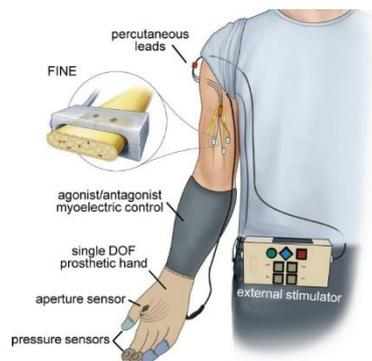
Figure 1: schematic diagram of a Home system for sensory restoration [6].
