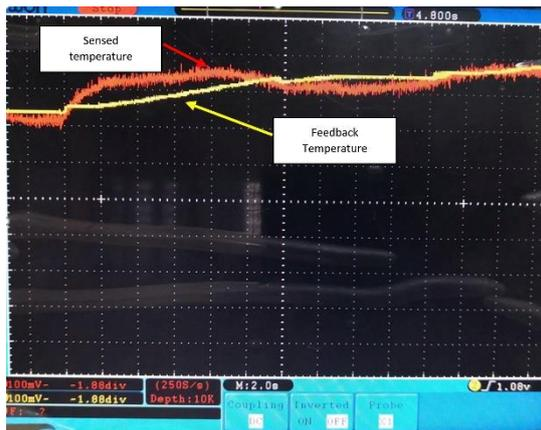
Figure 8. response for fast rabid change in the reference signal from 45-55-50 Celsius.
