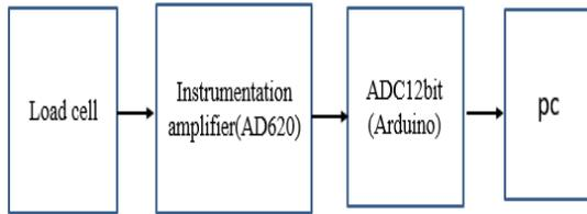
Figure (3). Schematic of basic system block diagram..
