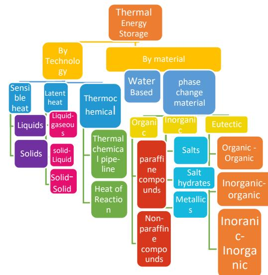
Figure 1: Classification of different types of energy storage
