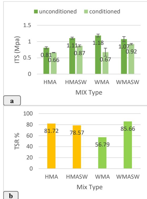
Fig. 5 Indirect tensile strength properties of mixtures (a- In direct tensile strength and b- Tensile strength ratio)
