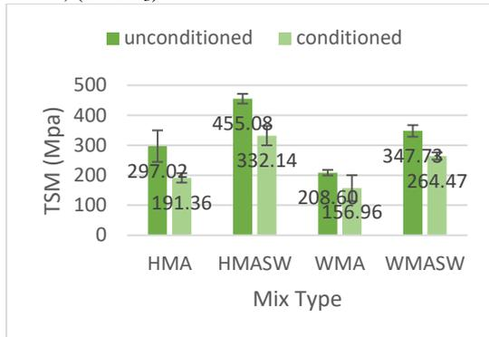
Fig. 6 Tensile Stiffness Modulus of mixtures
