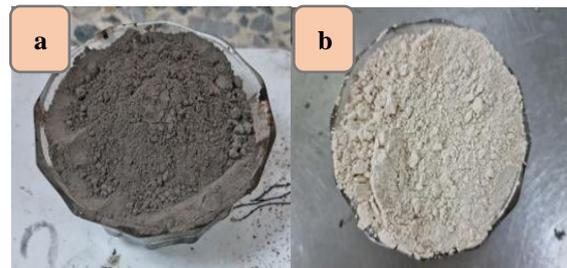
Fig. 2 The two types of fillers, a- CaCO<sub>3</sub> filler and b- Sulfur waste filler.
