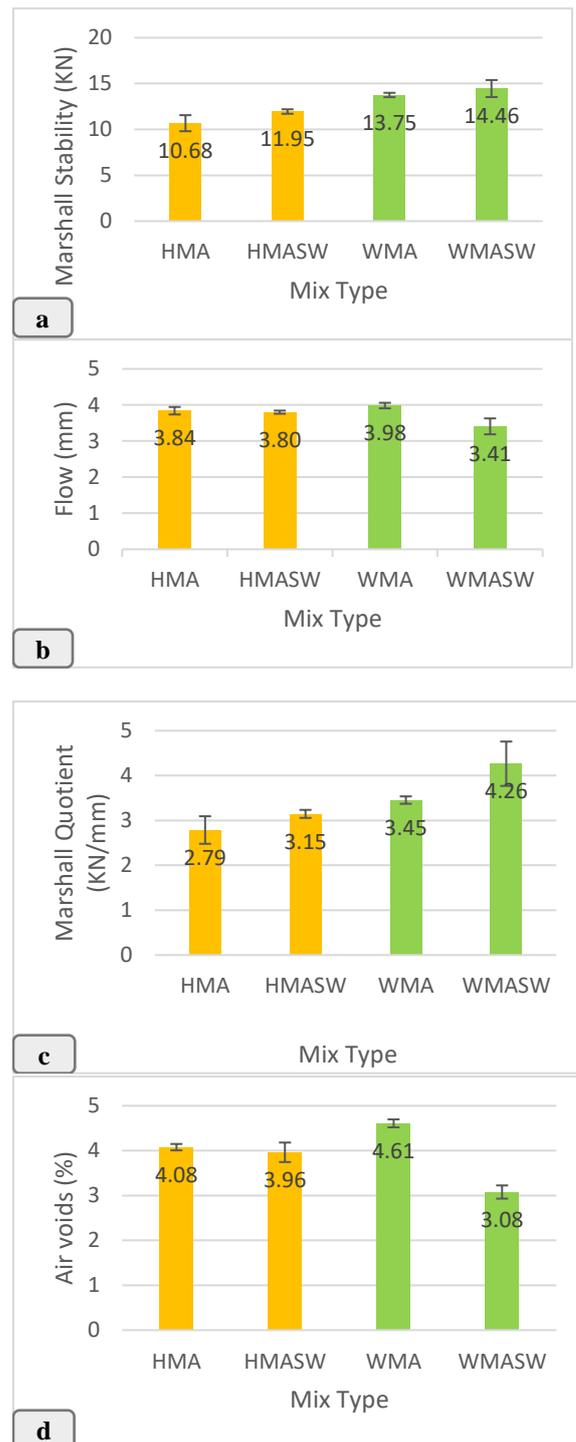
Fig. 4 Marshall properties of mixtures (a- Marshall stability, b- flow, c- Marshall quotient and d- Air voids)
