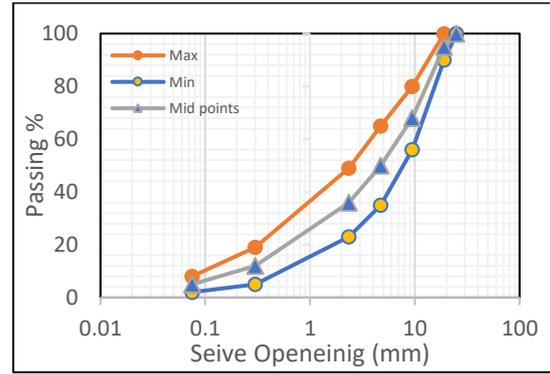
Fig. 3 The Gradation of the Mixtures
