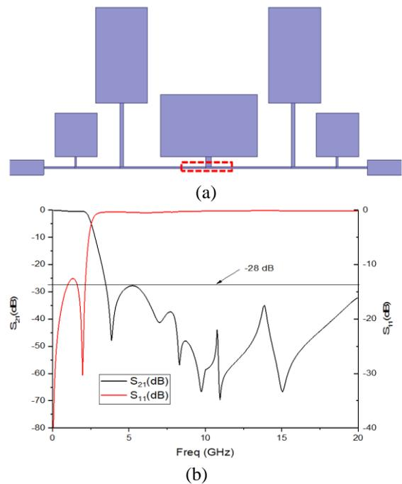
Fig. 6 (a) Top view of the 11<sup>th</sup> generalized Chebyshev microstrip LPF with DGS (b) Simulation of the frequency response of the 11<sup>th</sup> generalized Chebyshev microstrip LPF with DGS.
