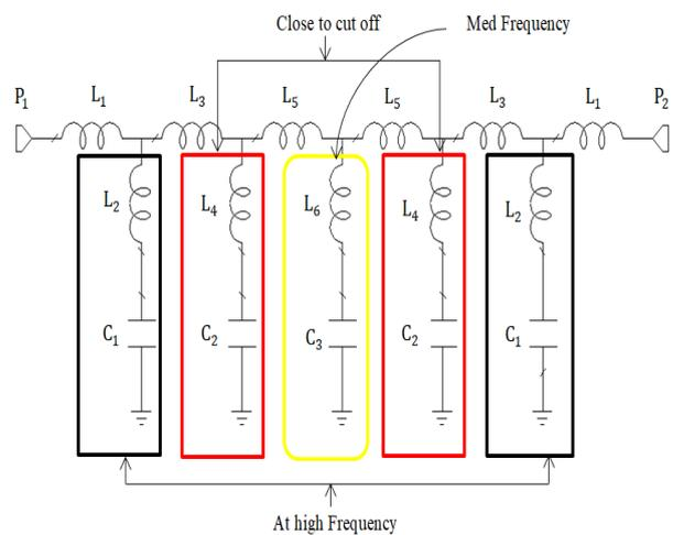
Fig. 1 LC equivalent circuit of 11<sup>th</sup> generalized Chebyshev LPF.
