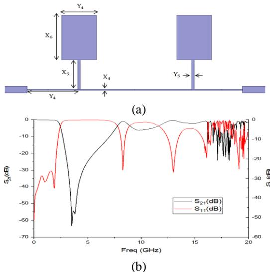
Fig. 3 (a) Top view of microstrip LPF with two TZs closed to passband (b) Simulation of the frequency response of two TZs closed to passband.
