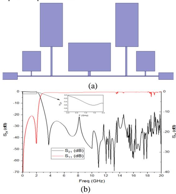
Fig. 5 (a) Top view of the 11<sup>th</sup> generalized Chebyshev microstrip LPF (b) Simulation of the frequency response of the 11<sup>th</sup> generalized Chebyshev microstrip LPF.
