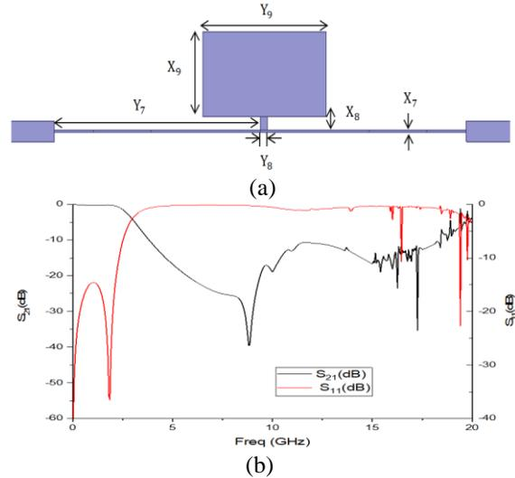
Fig. 4 (a) Top view of microstrip LPF with one TZ at moderate frequency (b) Simulation of the frequency response of one TZ at moderate frequency.
