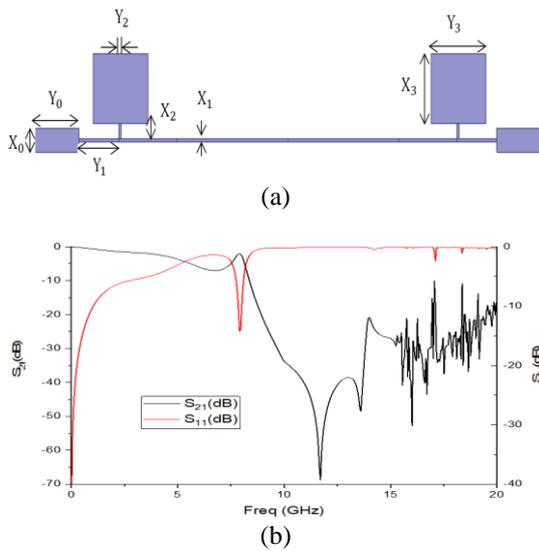
Fig. 2 (a) Top view of microstrip LPF with two high TZs (b) Simulation of frequency response of two high TZs.
