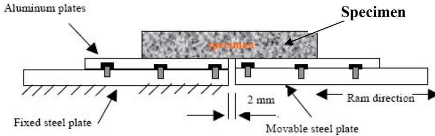
Figure (3), Concept of the Overlay Tester [16].
