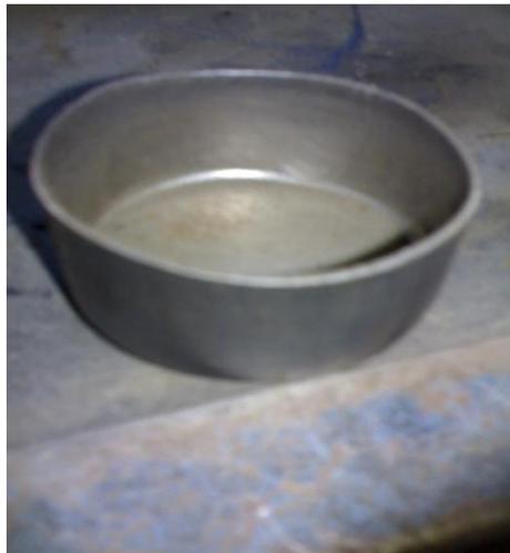
Figure (2) the sample of completely drawn cup
