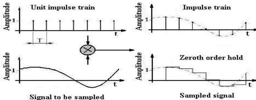
Fig. (5):- The comparison of sampling between Unit impulse train and Zero order hold
