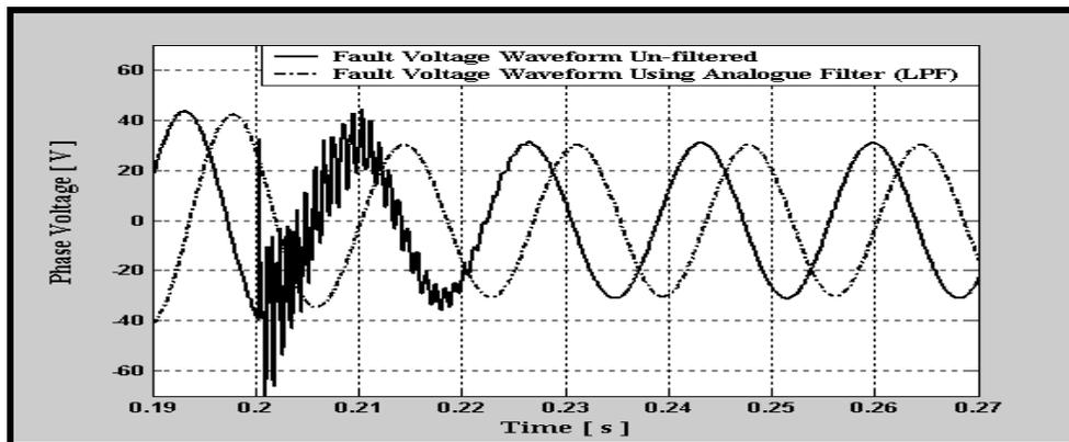
Fig. (8):- Voltage waveforms of fault using anti - aliasing filter at fault inception =  $-90^\circ$  and fault location = 50 %
