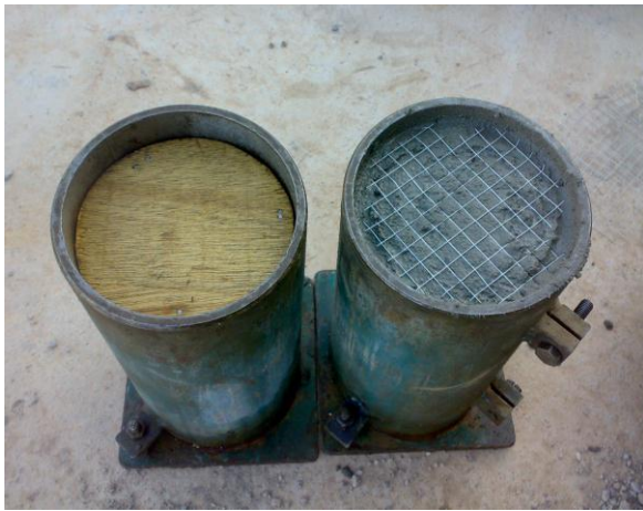
Figure ( 1 ) : The mould used for casting disc specimens and wire mesh layer arrangement .
