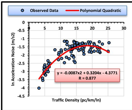
Fig. 5: Effect of Traffic Density on the Transformed Acceleration Noise on Multi-Lanes Arterial Roads
