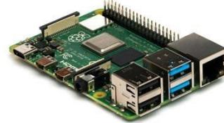
Fig (10) Raspberry Pi board
