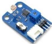
Figure (15) Intensity Illumination sensor
