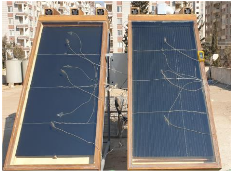
4a conventional SAH 4b improved SAH. Fig. 4. Experimental rig
