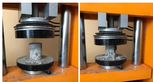
Fig. 6 Sample testing to determine the compressive strength
