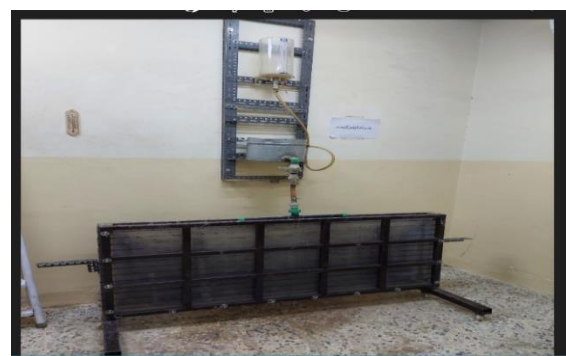
Figure 1: Soil container and water processing system
