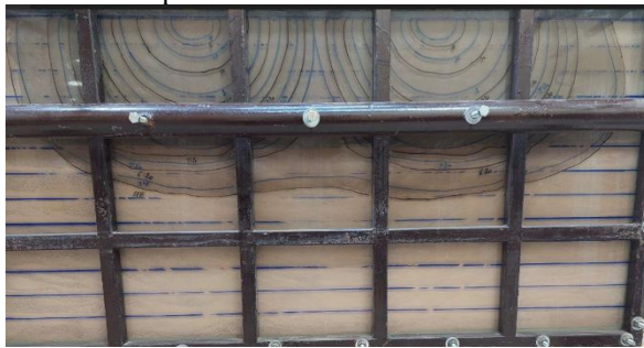
Figure 6: Wetting pattern in a layered soil (sandy loam in the upper layer and clay in the lower layer) with application rate 0.956 \text{ cm}^3/\text{min}/\text{cm} and 50 cm distance between two drips
