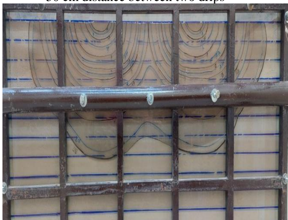
Figure 7: Wetting pattern in a stratified soil (clay over sandy mixture) with application rate 0.956 \text{ cm}^3/\text{min}/\text{cm} and 50 cm distance between two drips
