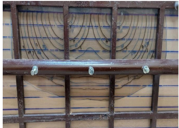
Figure 8: Wetting pattern for a layered soil (sandy loam over clay) with application rate 1.515 \text{ cm}^3/\text{min}/\text{cm} and 30 cm distance between two drips
