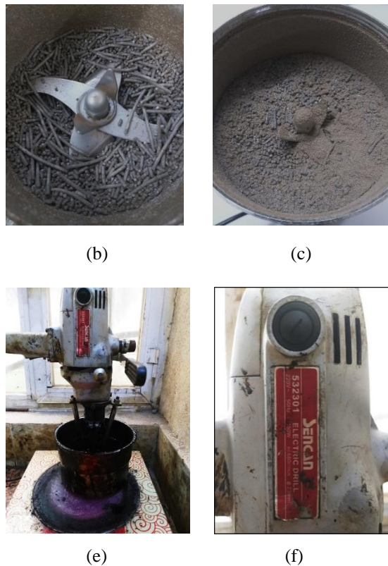
Fig. 4 Mixing ABS and AC (a-ABS filaments, b-ABS filaments during grinding, c-ABS filaments after grinding, and e-details of the shear mixer utilized in the ABS mixing process).
