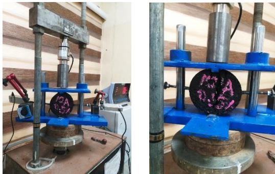
Fig. 8 ITS (a- Automatic multi-tester machine with ITS equipment and tested specimen, b- Specimen after failure).
