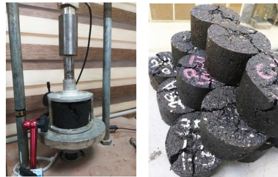
Fig. 7 Kim test (a-Automatic multi-tester machine with Kim equipment and tested specimen, b-Specimens after failure).
