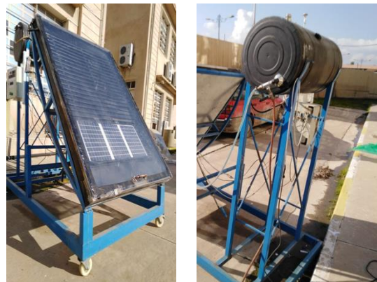
Fig.1 photovoltaic thermal collector used in the current study.
