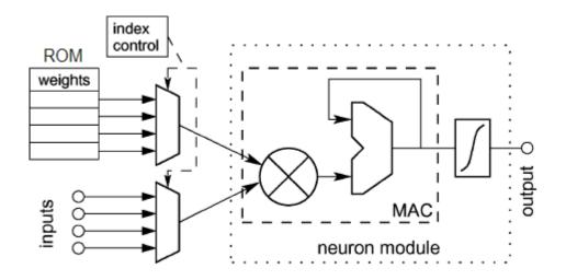
Fig. (2), Neuron structure—serial processing.
