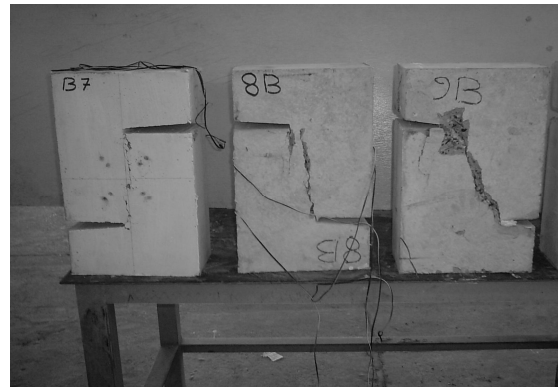
Fig.(18) Mode of failure for B(7,8,and 9)
