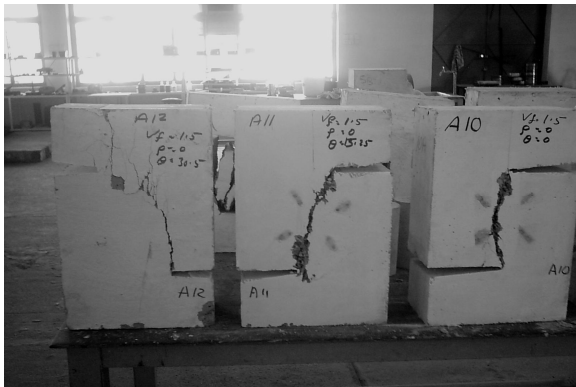
Fig.(17) Mode of failure for A(10,11,and 12)
