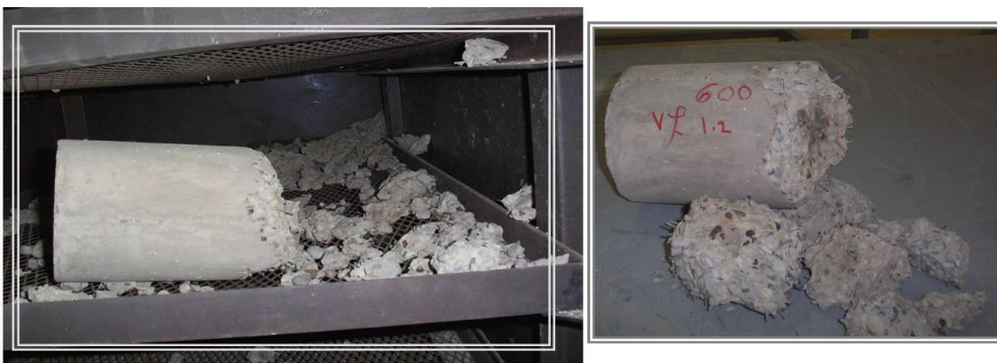
Fig. (12) Explosive spalling
