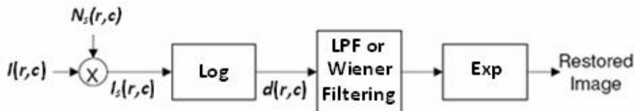
Fig. 1 A signal flow diagram of a typical homomorphic transformation.
