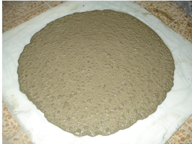
Figure (9): Measurement of slump flow (mix2)
