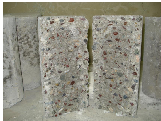
Figure (12): Linear Failure of cylinder
