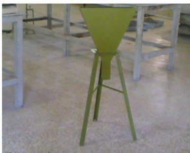
Figure (4): V-funnel apparatus
