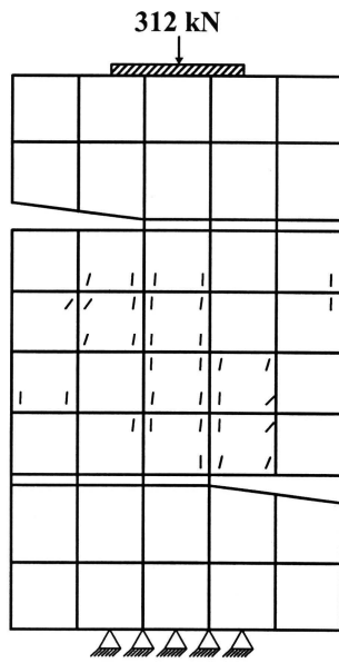
Fig.(12) Cracks pattern of specimen A2, V_f=0
