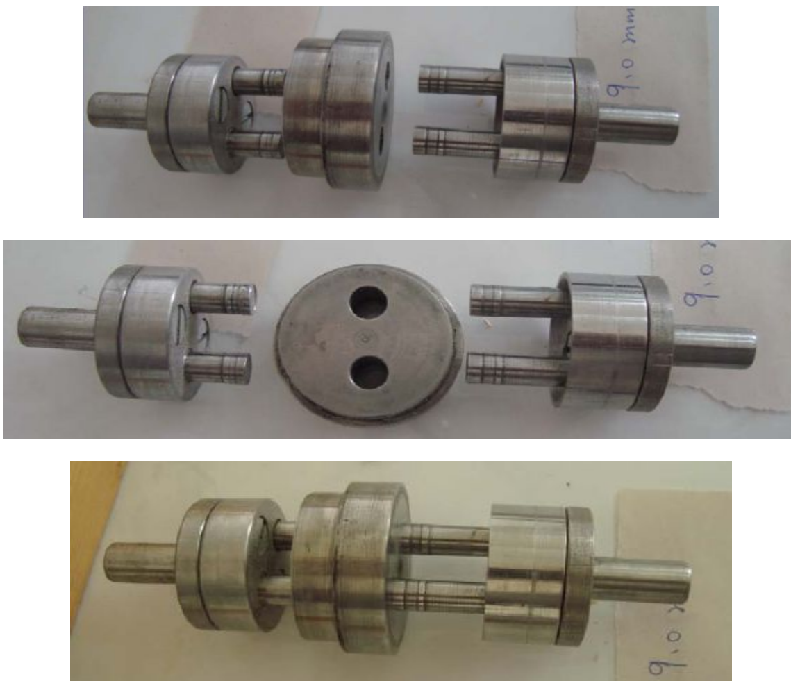
Figure ( 12 ) A new manufactured upper , lower punch and Die of size (9 mm)
