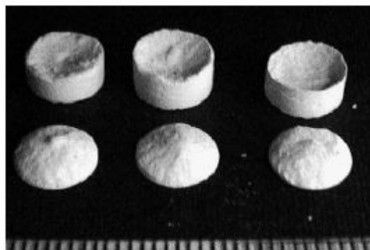
Figure (9) photography of broken tablets upon ejection
