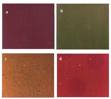
Fig. 7 Photomicrographs of SWMABs (a = 0.0%, b= 3% SWMAB<sub>1</sub>, c=5% SWMAB<sub>1</sub>& d=3% SWMAB<sub>0</sub>)
