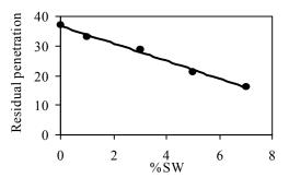
Fig. 5 Residual penetration of SWMAB<sub>1</sub>
