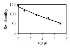
Fig. 2 Ductility of SWMAB<sub>1</sub>
