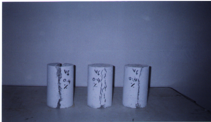
a. Splitting test V_f = 0.4\%
