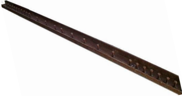
Plate 3: The steel channel with its attached headed studs for beam TB-NU45/90 .
