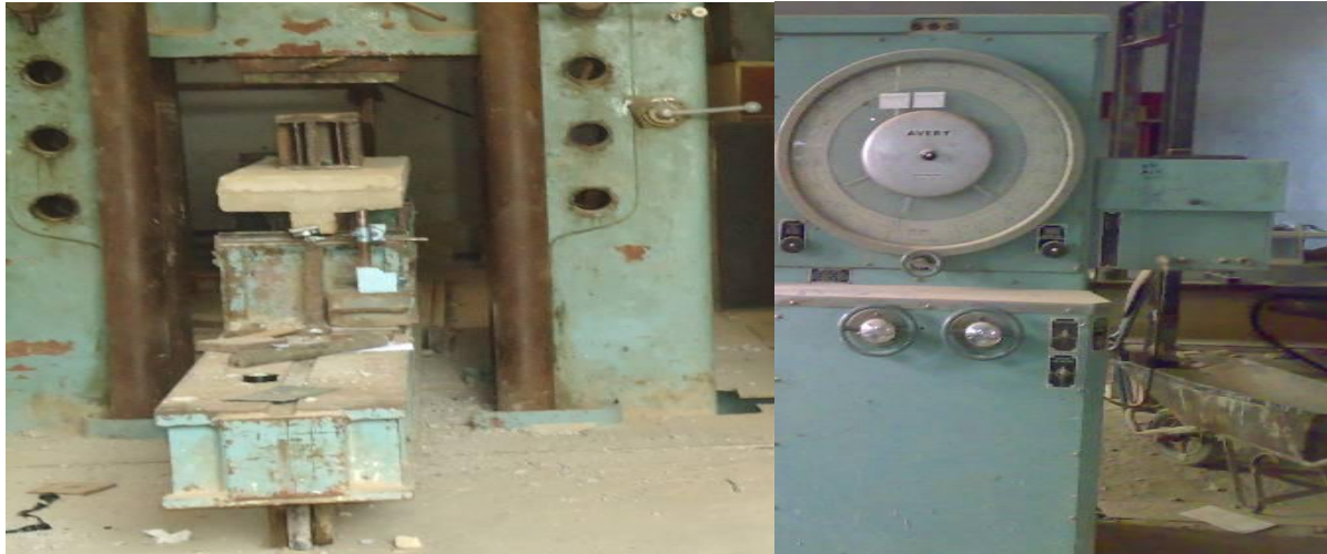
Plate 5: The universal testing machine (8551M.F.L.system) with a typical test beam
