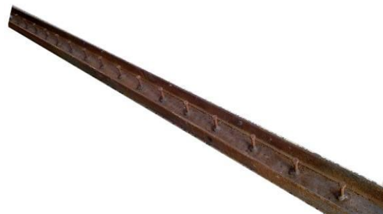
Plate 2: The steel channel with its attached headed studs for beam TB-U90 .
