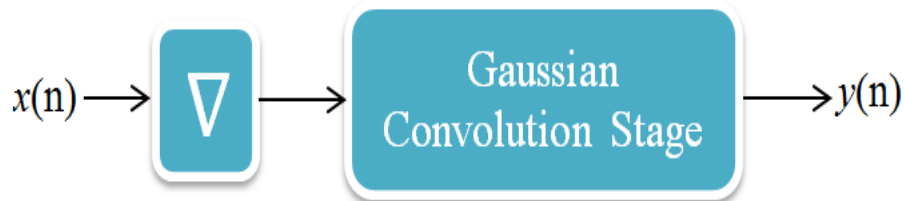
Fig.2A proposed system with Gaussian function and a derivative stage.
