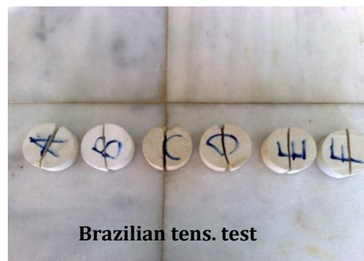
Figure (3): Failure of specimens rocks in mechanical tests
