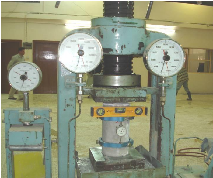
Figure (13) Modulus of elasticity test
