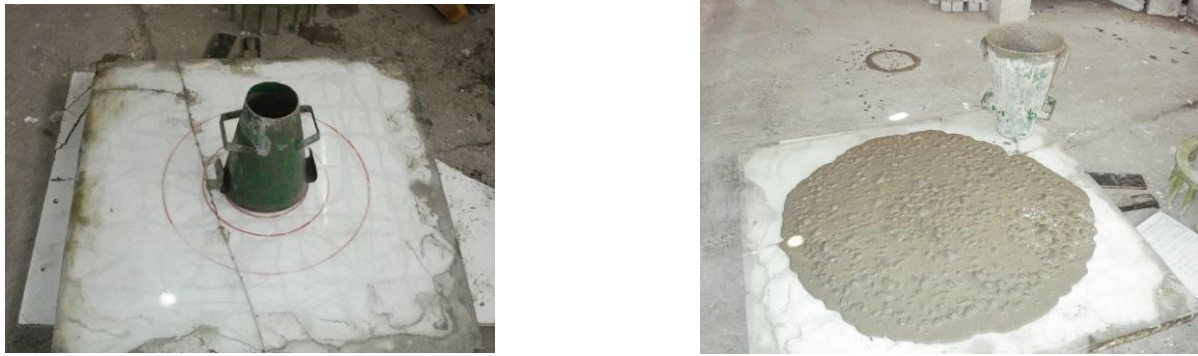
Figure (1) Slump flow test
