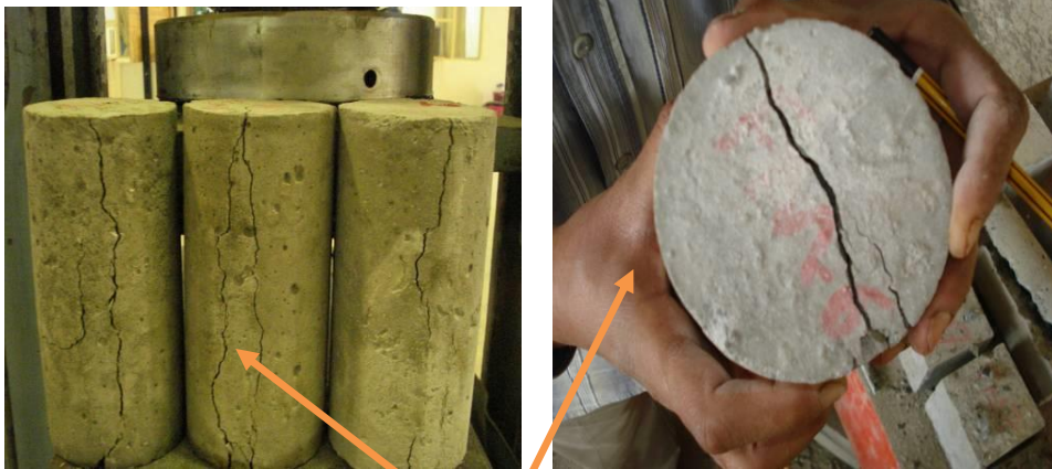
Failure in the splitting test
