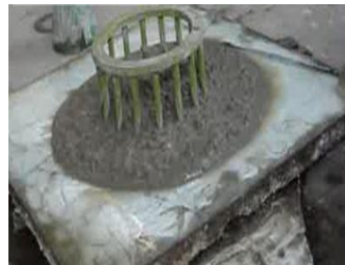
Figure (2) J-ring test
