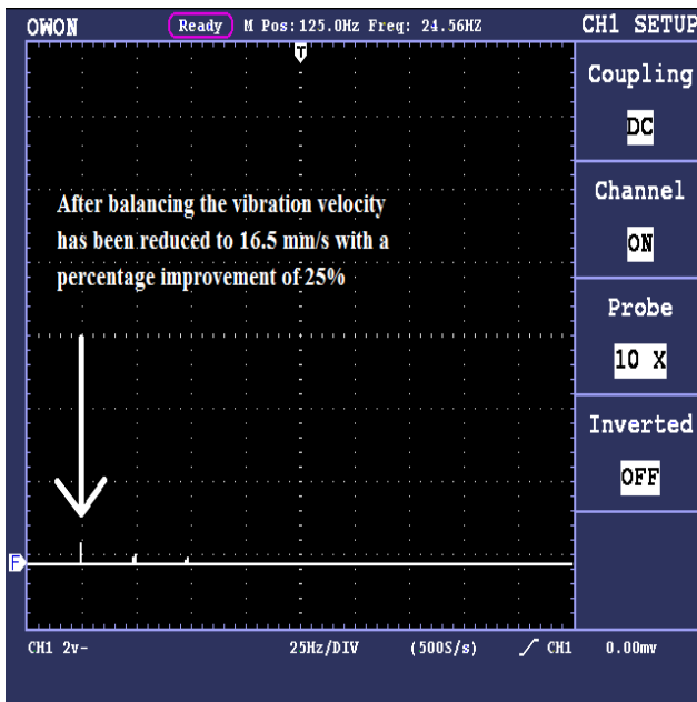
(5c). After balancing using three test runs method
