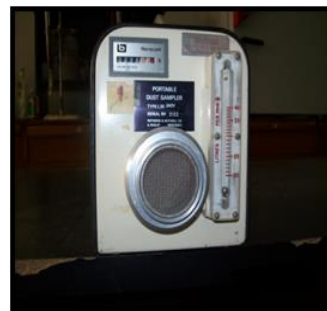
Figure (2), drawing air equipment to collect PM type Sniffer
