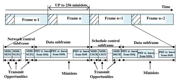
Fig.(2): frame structure in the mesh mode
