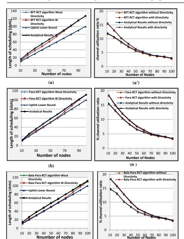
Fig. (10): shows the relationship between the length of schedule (a,b.c) and the channel utilization ratio (a',b',c') against the number of nodes for BFT, Para and Bala-Para RTCAs with and without directivity when the traffic demand is unified
