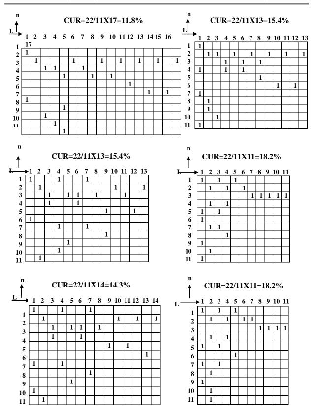
Fig.(9): slot assignment using Relay Model Scheduling with NS criteria (a), (b), (c) without and (d), (e), (f) with directivity for BFT-RTC, Para-RTC and Bala-Para-RTC algorithms respectively
