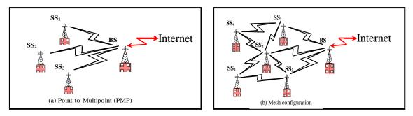
Fig.(1): WiMAX PMP network and mesh network
