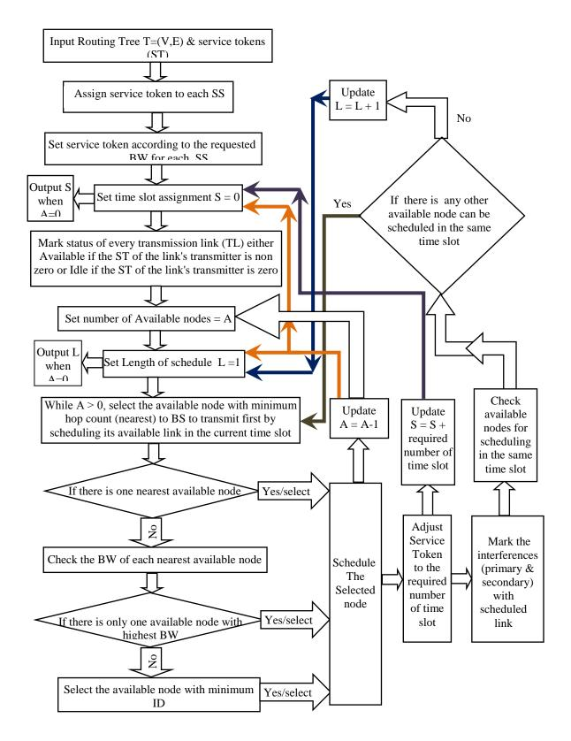
Fig.(8): Flow chart of the proposed scheduling algorithm
