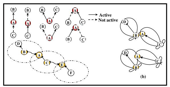
Fig.(3): shows interferences (a) primary and secondary interferences without directivity (b) places where secondary interferences could happen when directivity introduced.
