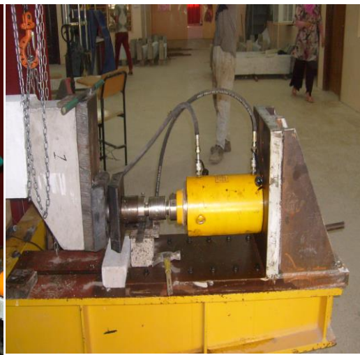
Figure (5) Set up of Jacking.
