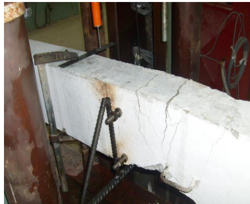
Figure (7) Failure of Control Column
