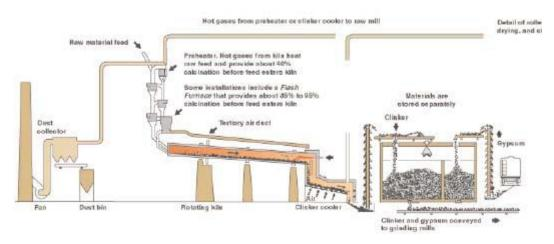
Fig. (3): Schematic of a dry kiln
