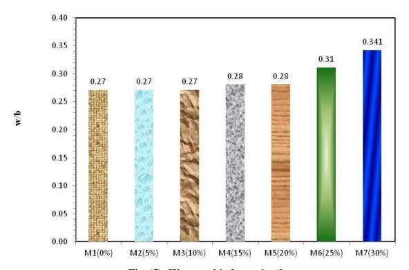
Fig. (5): Water to binder ratio of cement pastes
