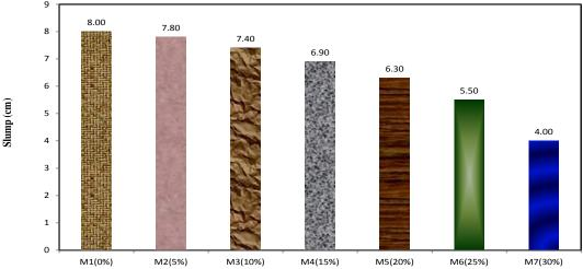
Fig. (9): Slump results of concrete mixes
