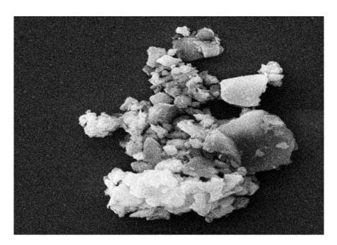
Fig. (4): Scanning electron microscopy of the particles of (CKD)
