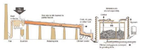
Fig. (2): Schematic of a wet kiln
