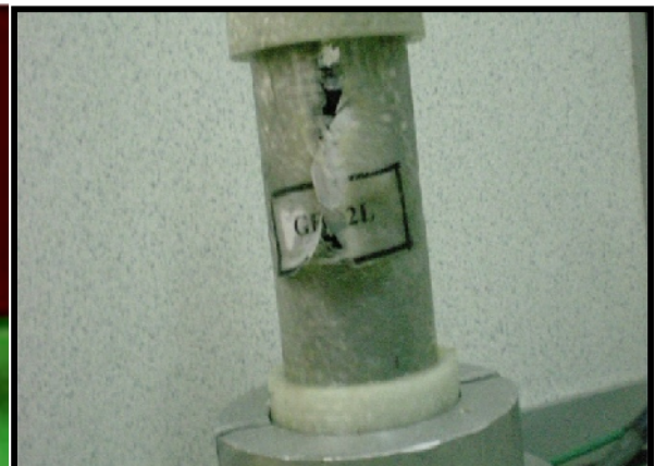
Fig. 5: The specimen after failure occurred
