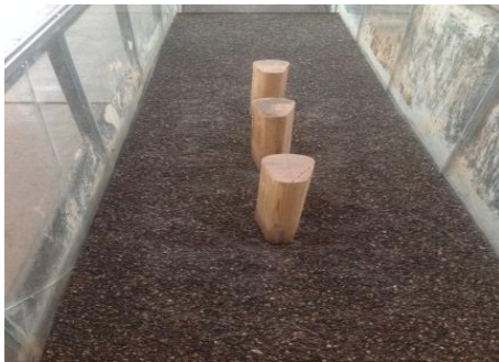
(b) Scour bed around the group of bridge piers 4-10 cm.
