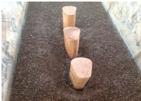
(c) Scour bed around the group of bridge piers 6-10 cm.
