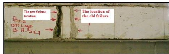
Fig.10 The rehabilitation of the prism after failure
